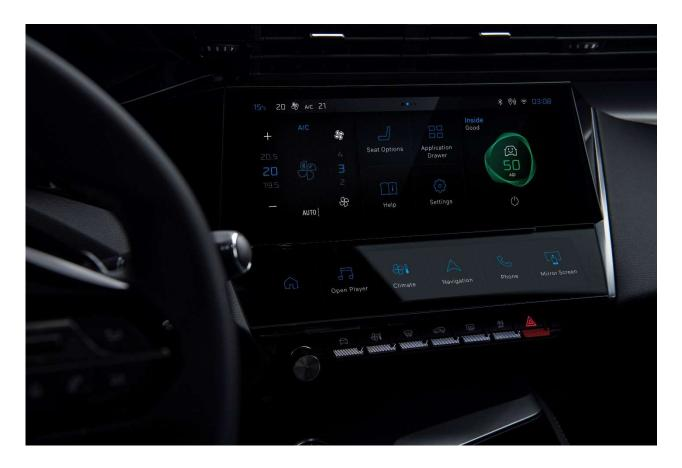
At the top of the screen, a permanent banner displays outdoor temperature information, air conditioning, position in widget pages, connectivity data, notifications and time.
