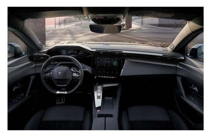
The construction of the dashboard of the new PEUGEOT 308 SW is based on a "high wind" architecture which places the air vents directly in front of the occupants' heads. This position is optimal for driver and passenger comfort.
